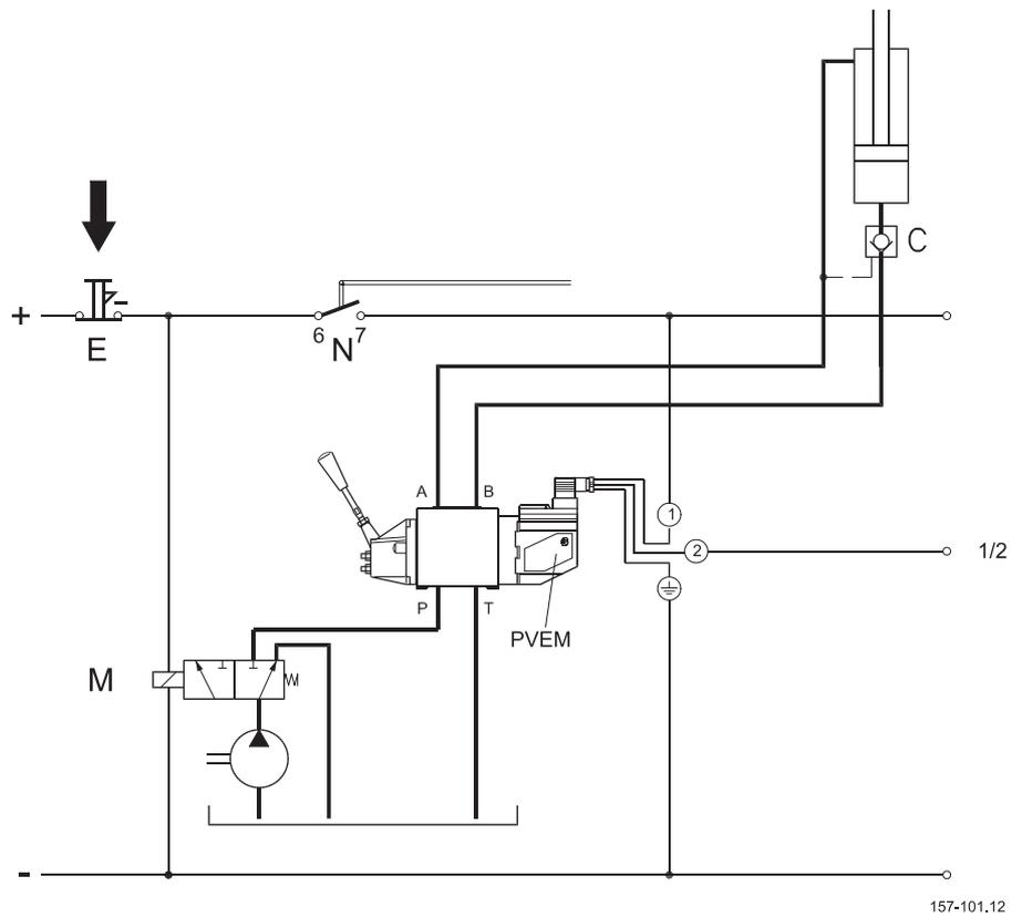
The difference between this safety method and the one previously described (1) is that here there is no built-in automatic fault monitoring and a neutral position switch (N) is connected. The method still gives a high degree of protection, but requires operator intervention. It is recommended that the neutral position switch be always connected to the electrical system. This then automatically cuts off current to the proportional valve when the remote control unit is in neutral position.
