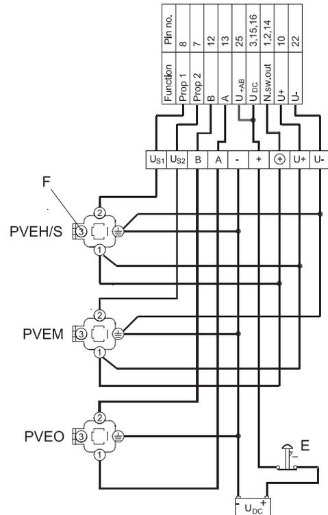
F: Signal output, fault monitoring
