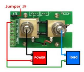
Figure 2-4 Two-wire wiring diagram
