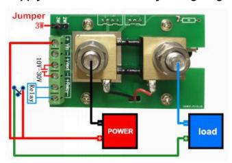
Figure 2-6 Three-wire connection Relay wiring diagram
